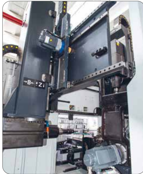
Auxiliary axes with 11-3/4" stroke
